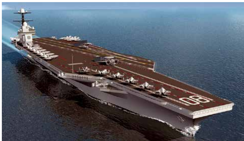
The USS Gerald R. Ford, the Navy’s next-generation $13 billion aircraft carrier, is a pioneer in many ways: It’s the first of its kind to be designed by using a full-scale digital 3D model. It will save more than $4 billion in total ownership costs during its 50 years of service and operate effectively with 700 fewer crew members than its predecessor.
